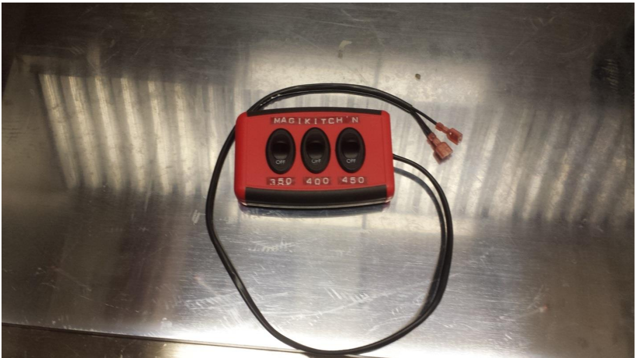
Figure 8: Now that the panel is lowered you can use the MagiKitch'n Solid State Thermostat Calibration Tool to calibrate the controls. Verify that all switches are in the 'OFF' position.
