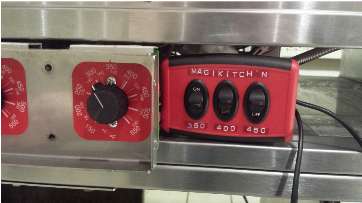
Figure 10: Flipping up the front panel to show the control knobs, switch the 350°F toggle into the 'ON' position. Burners should not ignite until 350°F is reach on the control knob.
