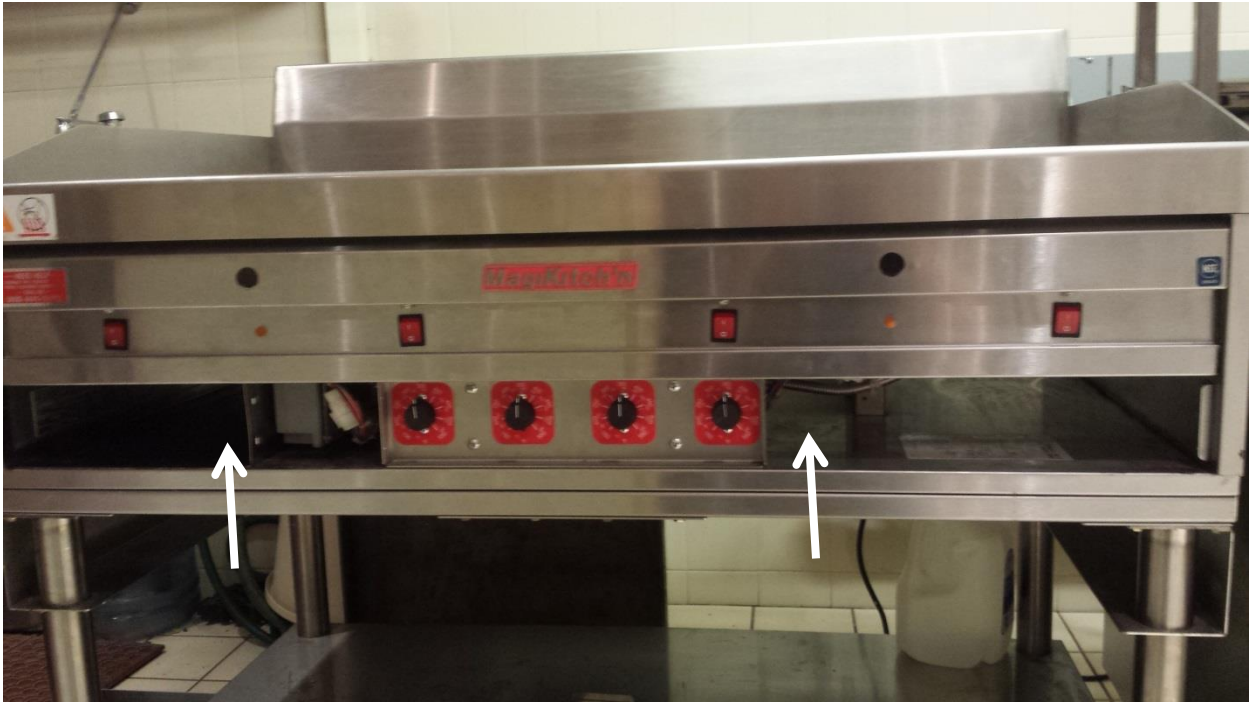
Figure 5: Remove front Left and Front Right panels.
