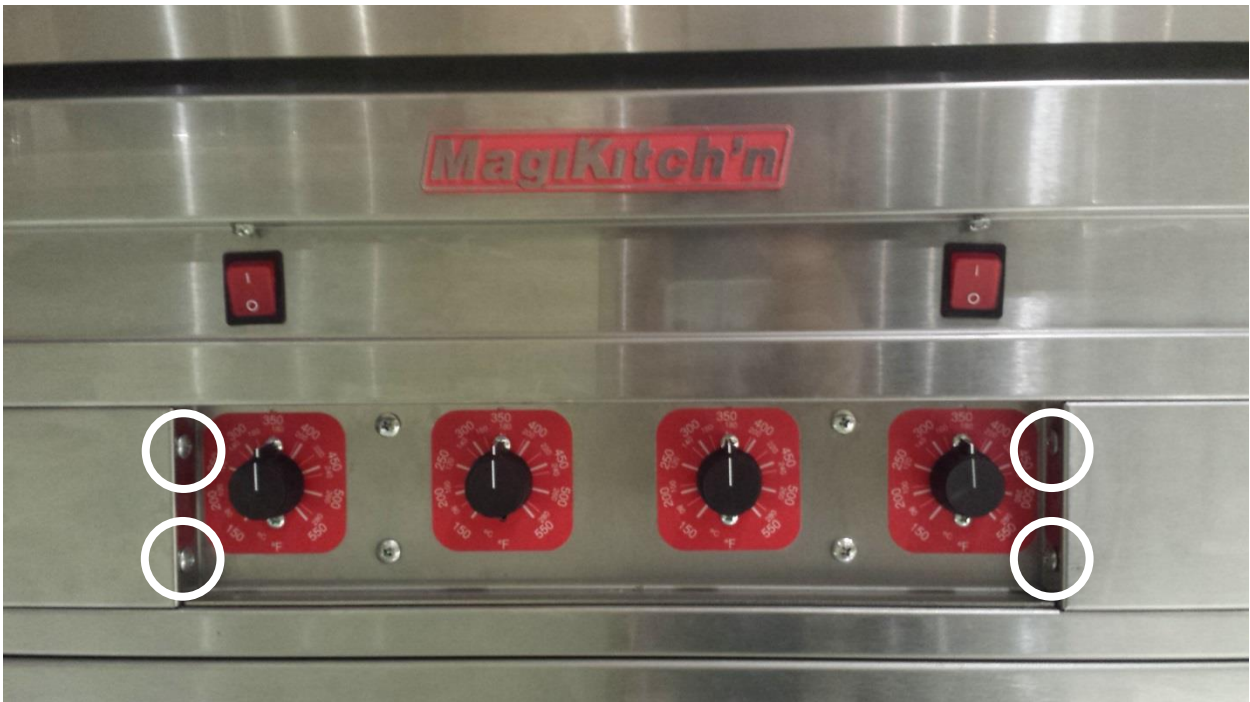
Figure 4: Next remove the four (qty. 4) Philips head screws, which will allow you to remove the front Left and front Right panels.
