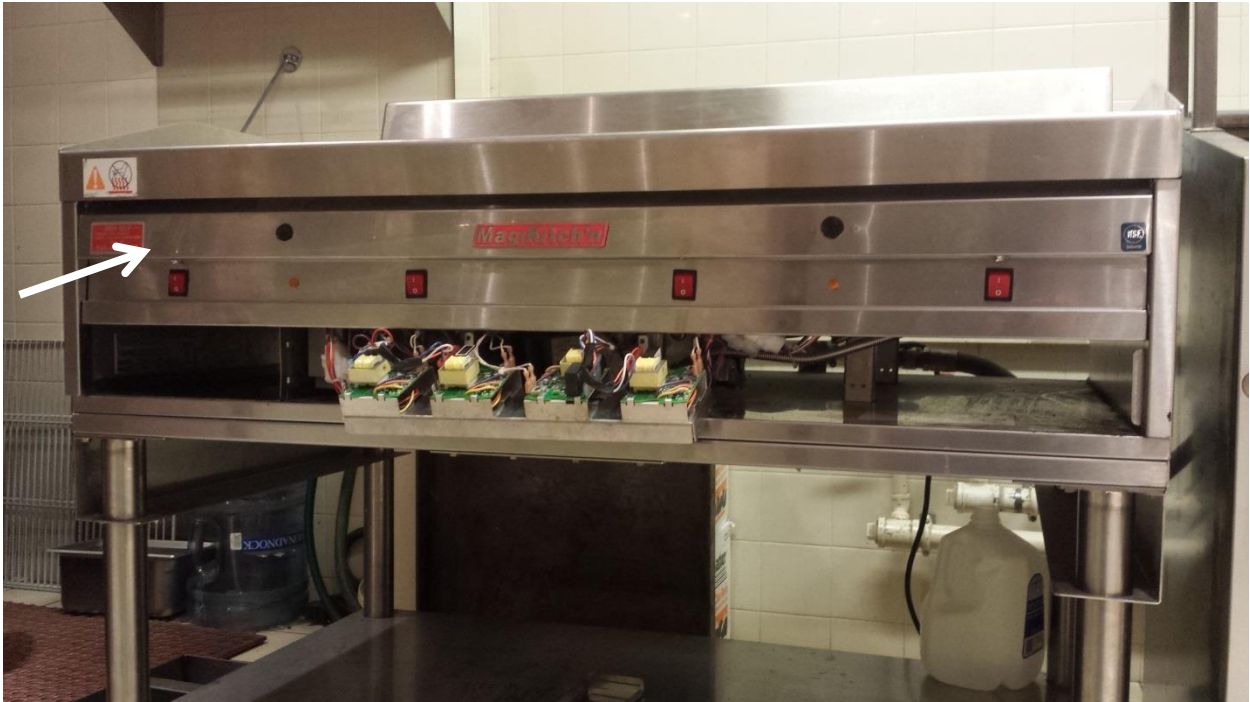
Figure 7: The front panel (indicated with arrow) will need to be removed to be able to lower the Solid State Thermostat Control Panel, as shown above. Once removed, replace two (qty. 2) 3/8" hex head self-tapping screws for ease of testing.
