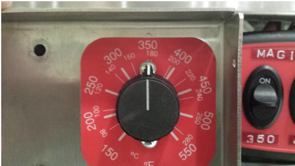
Figure 11: With the 350°F Test Switch in the 'ON' position, as well as the units 'ON/OFF' switch in the 'ON' position turn the control knob until the unit turns on and burners ignite. Go beyond the temperature indicated on the test controller, and then slowly back to the temperature on the switch. When the control knob is on the left side of the line, as shown above, the unit should be off, indicating that the unit is at the indicated temperature already. When the control knob is on the line of the indicated temperature or to the right of the desired temperature, the unit should re-ignite the burners and come to the proper temperature.
