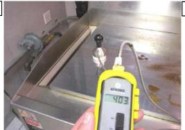
When the calibration of the control is satisfactory, tighten the ferrule nut completely
