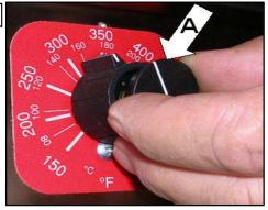
Replace the knob cap so that the indicator lines are aligned with each other.
