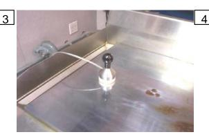
Place a weighted griddle temperature probe on the cooking surface 9-12" from the front edge of the griddle plate.
