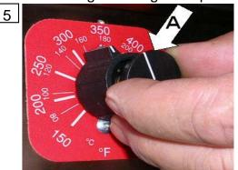
While the Unit stabilizes at Temperature for 30-60 minutes, remove the contol knob caps
