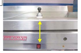
Align the griddle probe with the power switch for the cooking zone being calibrated.
