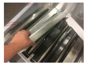
If the burners or pilot runner tube have debris build up on them, use a wire brush to remove the build up. If the ports of the burner are clogged, use a sharp instrument to clean the ports.
