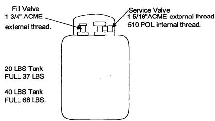
NOTE: Some tanks are equipped with a single service valve with 510 POL threads.
